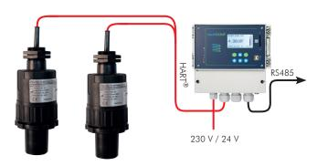
The MultiCONT multichannel process controller processes and displays measurement data supplied by NIVELCO's HART® equipped transmitters connected to a Multidrop loop. The transmitters (also mixed models) can be connected and remote programming can be also performed through the MultiCONT. Re-transmission of the data is possible via RS485 communication line to a PC or PLC when needed. The visualisation of the data can be done by NIVISION process visualization software.
