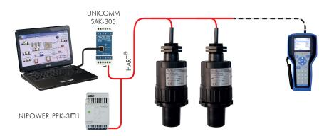
The instruments with HART® output can be connected to a PC using a UNICOMM SAK-305 HART®-USB modem. All measured values of the EasyTREK level transmitters can be visualized and/or the instruments can be remotely programmed via digital HART® communication. Applicable software for PC: EView2 configuration software or NIVISION process visualization software.
