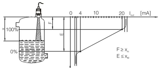
**ATTENTION!** When using off-site calibration, distance between the reflecting object and the unit must correspond to the required 4/20 mA values.
