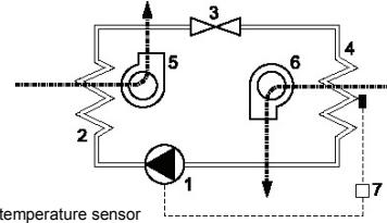
The compressor (1) compresses the refrigerant until high pressure is achieved. During this process temperature increases. In the condenser (2) heat is dissipated to ambient air, the coolant becoming liquid. The condenser fan (5) of the condenser takes ambient air through the condenser, then it releases the air.
