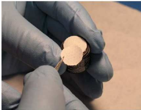
Figure 28 Installing Filter Media
