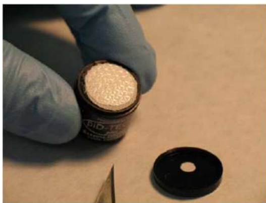
Figure 18 Removal of Filter Media
