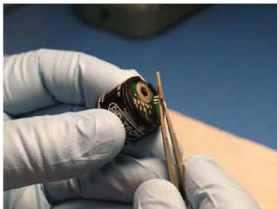
Figure 26 Cell Assembly installation
