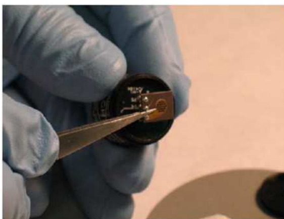
Figure 20 Removal of Cell Assembly
