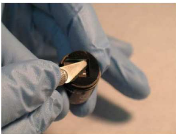
Figure 19 Removal of Spacer
