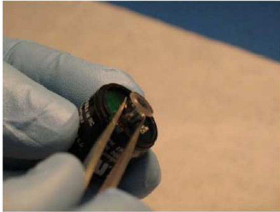
Figure 21 Removal of Lamp
